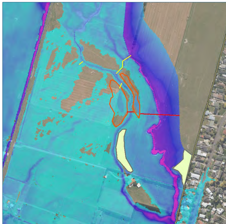
Figure 7 - Option 6 flood retention and diversion mechanisms
