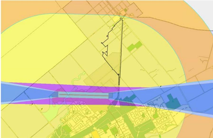
Figure 5-2: Freight Hub location in relation to the Airports Height restrictions (Yellow shows the area subject to the Horizontal surface control in R13.4.7.1)
