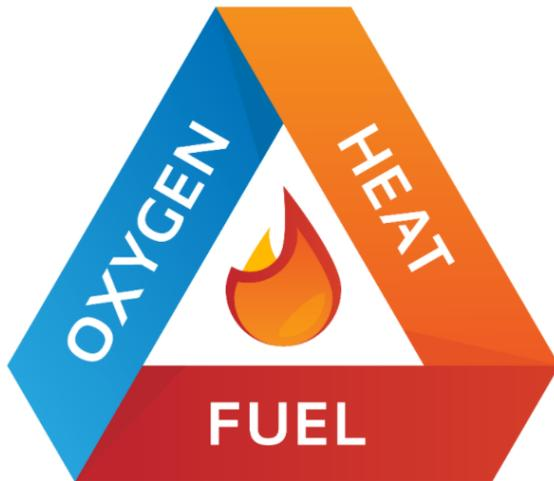
Oxygen is provided via the hearth fan through the breather holes in the floor. This seats the fire down low. When these holes block, the fire wants to climb the chimney to get oxygen. Heat or ignition source is provided by two burners directed downwards into the primary chamber. These also have fans generating oxygen. The gas involved is one fuel input. The bodies themselves are another.
