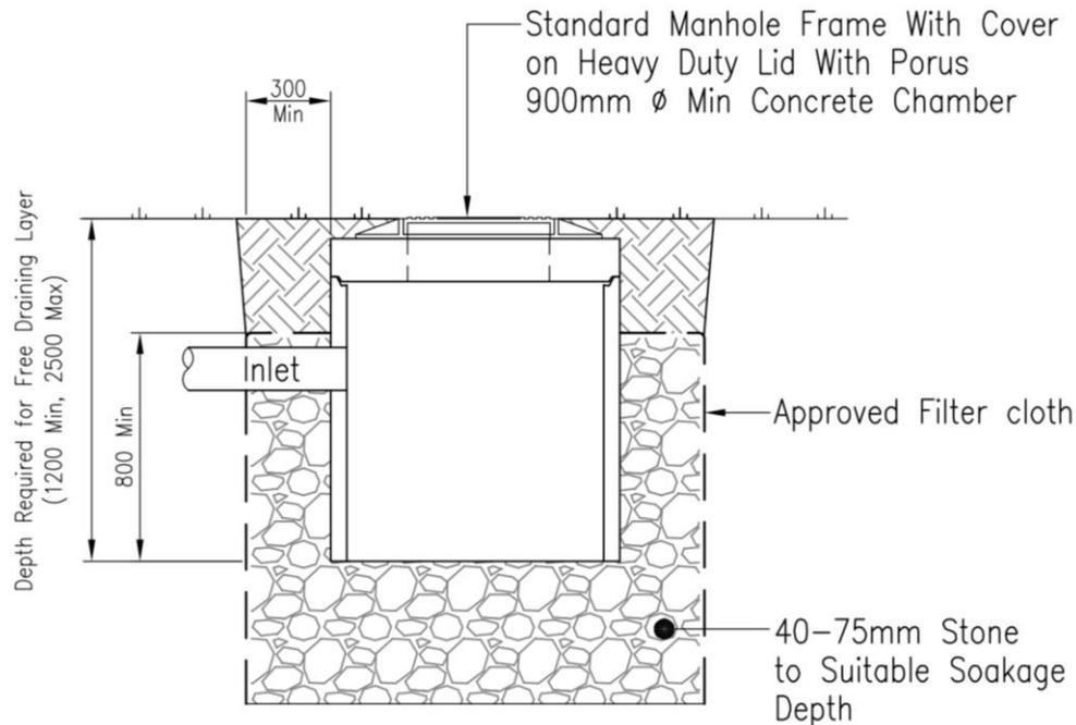
Figure 3: PNCC approved *standard soak pit detail*
