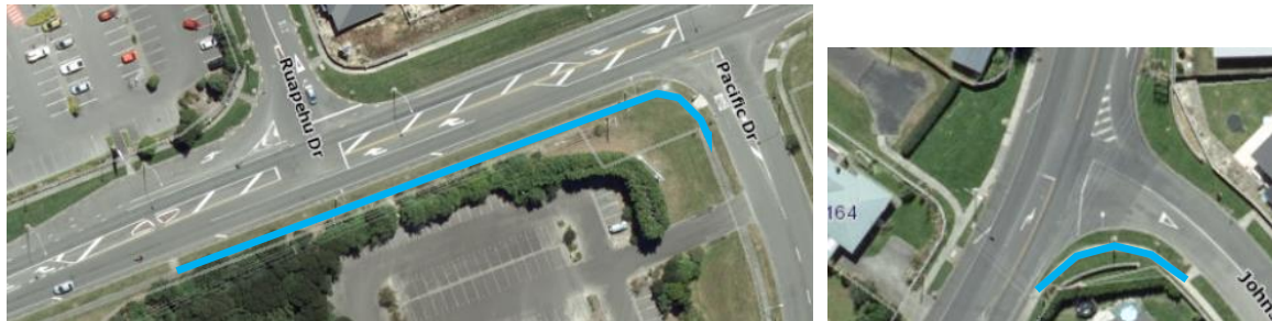
Figure 7: Possible Sections of Shared Path to Facilitate Right Turns into Side Roads for Cyclists
