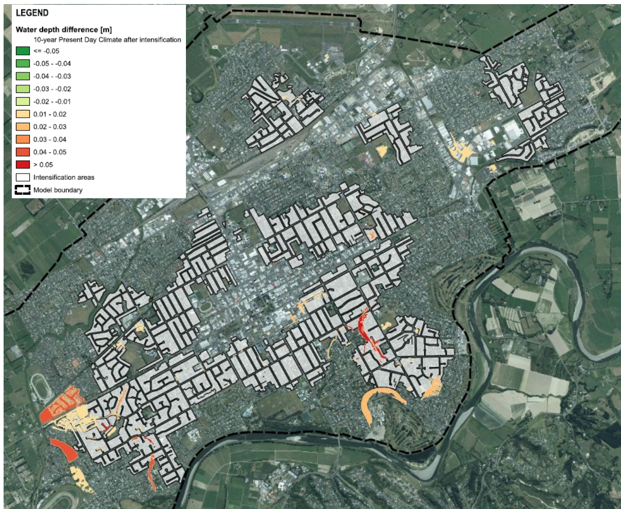
Figure 10: 1 in 10-year ARI flood depth difference due to intensification (Tonkin and Taylor, 8 May 2023)
