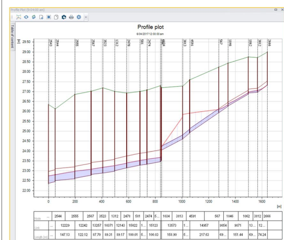
Figure 8: Existing 200mm pipeline on College street over long term with no upgrades 6
