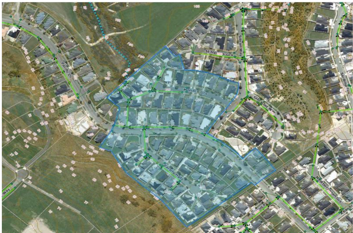
Figure 5: Stormwater Catchment discharging onto southern corner of the site
