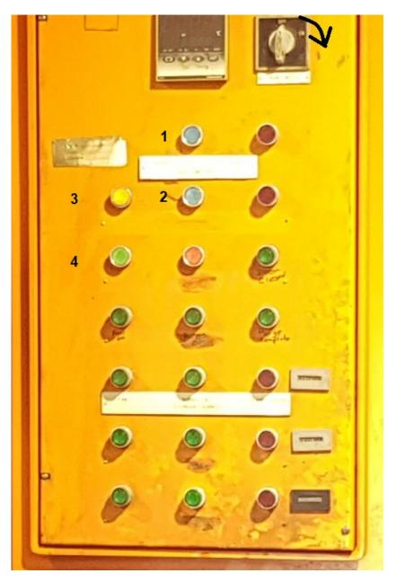
The hearth fan comes on for 5 minutes to clear the main chamber of any fumes that might ignite. The duration of this is set by the first timer.
