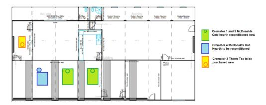
Figure 6: Proposed Cremation Facility with Locations of Cremators and Stacks
