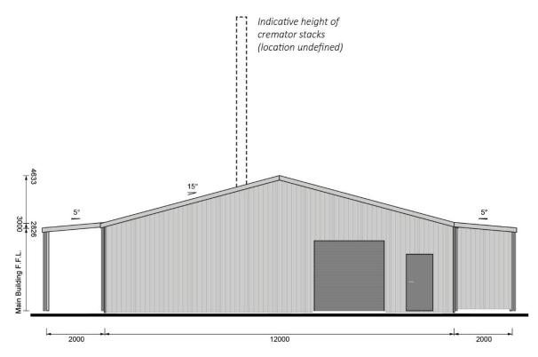
Figure 2: Elevation view of TotalSpan shed. Sourced from the Landscape Assessment. Note: the 10.5m high cremator stacks were excluded from this drawing so the height of these have been indicatively annotated.
