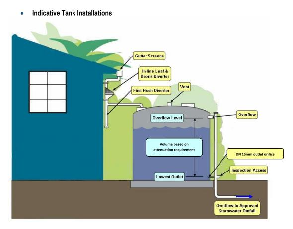
Figure 1: Above-ground detention tank – typical components (adapted to PNCC specific requirements from: *Three Waters Management Practice Note - HCC 06: Detention Tank*, Hamilton City Council)
