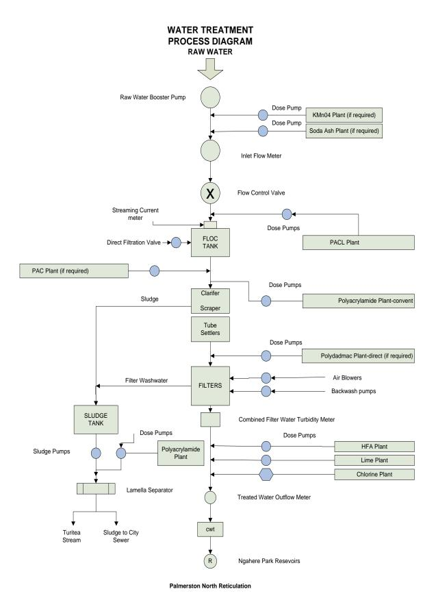
Figure 3 – Turitea WTP Treatment Process Flow Diagram
