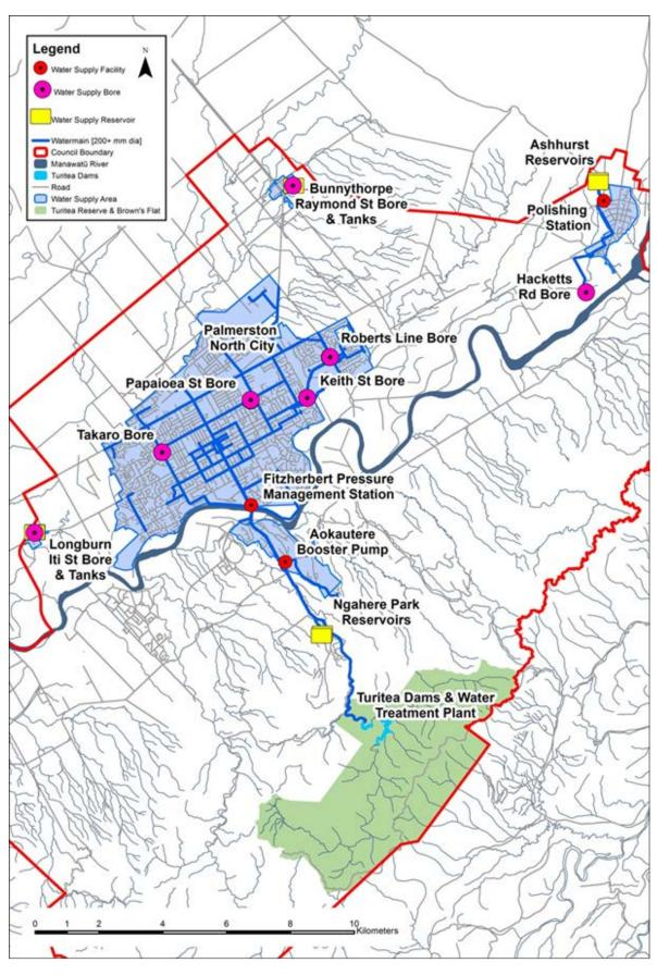
Figure 1 – Layout of Palmerston North Water Supply
