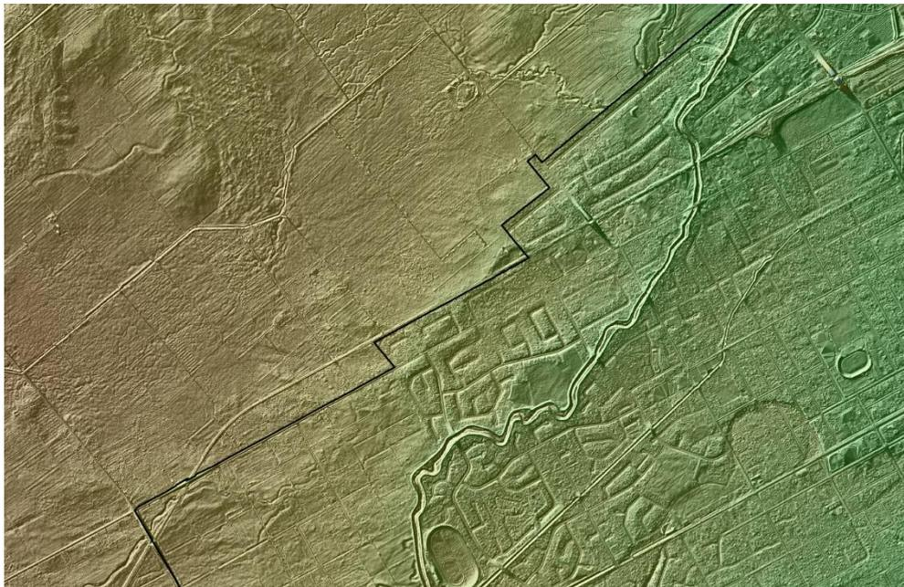
Figure 16 Detailed colour ramped DEM of the western part of Palmerston North City illustrating the presence and extent of levee-ed stream systems on this part of the Manawatu Plains. The main stream, Mangaone Stream, is contained behind man-made stop-banks. The trotting track is at the lower centre of the image.
