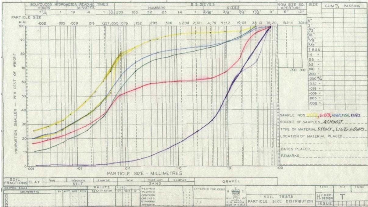
**3. Ashurst stony silt loam.** These grading curves indicate well graded soils with negligible liquefaction susceptibility.
